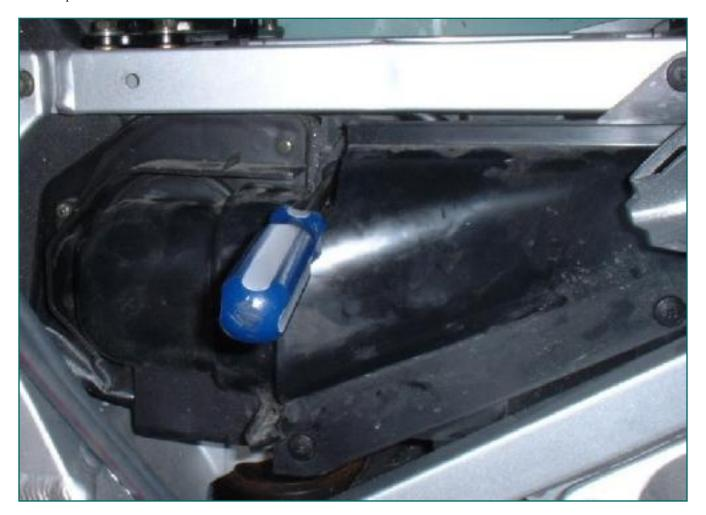
Next, remove the airbox cover. At least all 4 of these are the same 1/4 turn fastener. Unfortunately, the one indicated by the screwdriver is recessed and a PITA.
