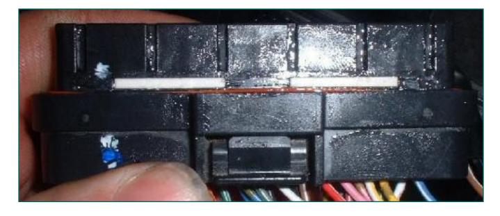
Put the plug in pin 27. Put the wire you removed in pin 25. Make sure they are fully seated and then re-lock the connector by pressing the left hand (as
