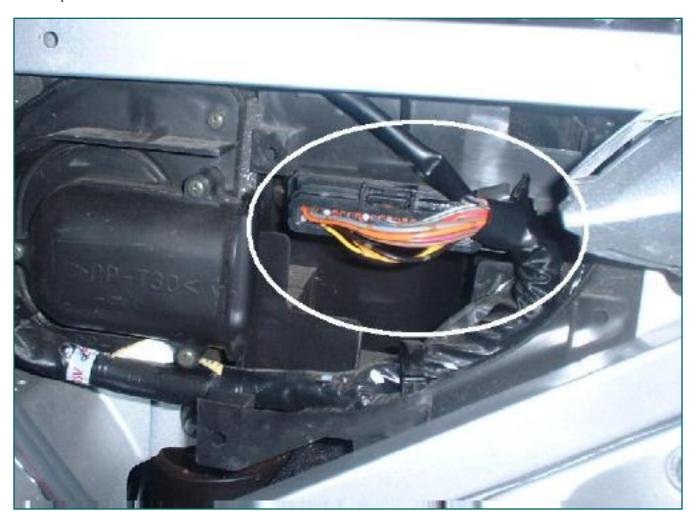
With the covers out of the way, the ECU is now accessible. Squeeze the black latch on the top of the connector as you pull it out of the ECU.
