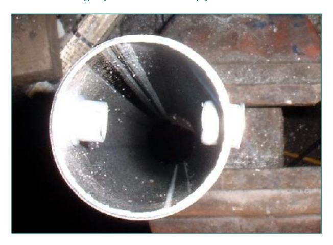
In an effort to reduce any possible restriction, I tried cutting 1/2 the threaded portion of a riv-nut off before installing it. The threads stripped out before it fully mushroomed, resulting in this failed installation on the right. The insert is loose, but cannot be removed and there are no threads left to seal it! The full threaded length is required to properly install the insert.
