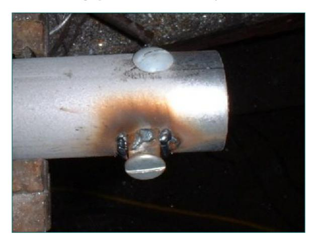
With all due respect to Yamaha, I offer this option which has no restriction to exhaust flow. I drilled a 33/64" hole in the pipe, threaded a bolt through a nut, inserted the protruding thread through the hole, and welded the nut to the pipe. The bolt can then be withdrawn and cut to length. For the real thing, spring for a stainless nut.
