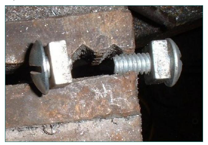
When cutting a thread, it's a good idea to temporarily install a nut first. Cut the thread off beyond the nut, then wind the thread past the end of the nut. If the thread binds while removing the nut, make sure the thread is not protruding past the nut and simply tap it against something solid to re-form the thread. In this case, because the bolt is now so short, it was easier to set it on the anvil of the vice and tap gently with a hammer.
