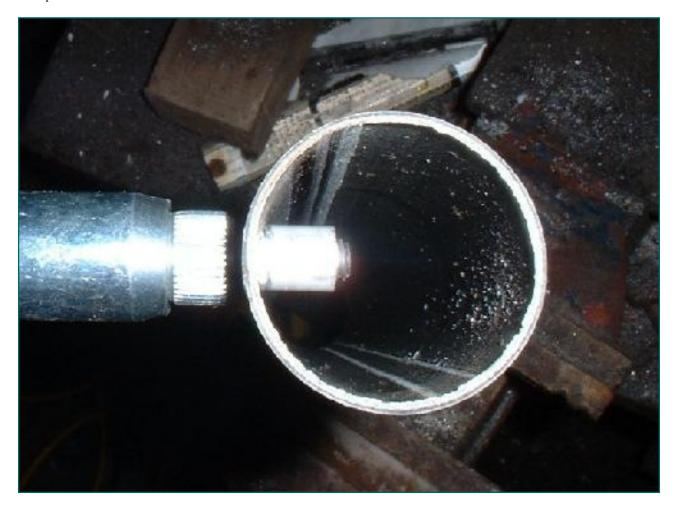
Here the riv-nut is assembled on the tool and inserted into the hole ready to go. One squeeze of the handle is sufficient. Attempting to compress the riv-nut further will only strip the threads. As described earlier, unscrew the tool from the insert using the removal knob.
