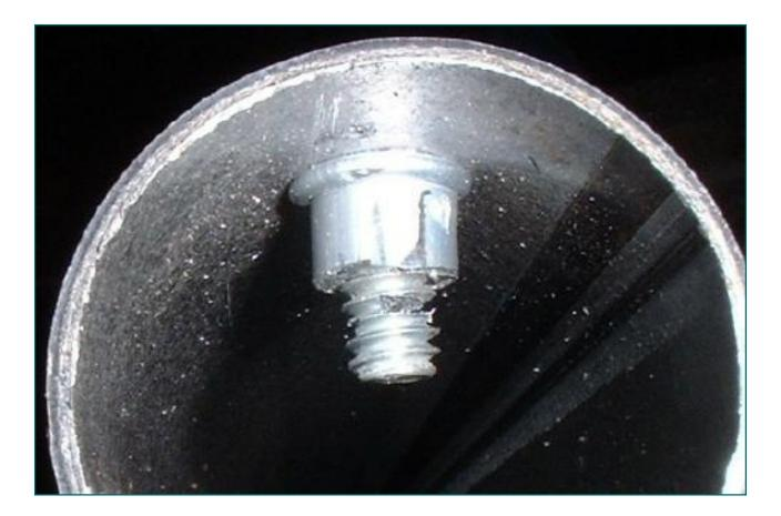
The hole is sealed with a bolt when not in use. As can be seen from this picture, the bolt may protrude into the pipe unless cut to length. Besides being a potential for further restriction, the exposed threads could become clogged with carbon deposits from the exhaust making future removal difficult or impossible. I suggest trimming the bolt to avoid problems.
