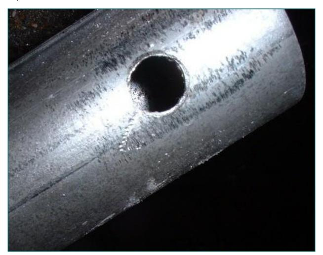
First a hole is drilled into the pipe where the port is required. European and Oceanic models have ports installed from the factory. Migmagal reports they are located "About 5 inches after the cylinder exits on each tube" and Woody concurs saying they are "about 125mm from the top of the exhaust ports". For clarity, these pictures are of a sample installed on a piece of scrap 1 1/2" exhaust pipe.
