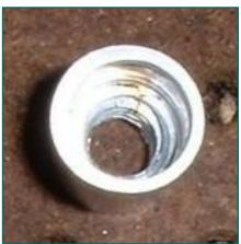
These are <u>riv-nuts</u> (or rivet nuts, or thread inserts depending on the manufacturer.) They are a hollow, threaded rivet that can be installed on the headers "blind" -- that is, without removing the headers. Yamaha instructs North American dealers to install these if it is necessary to check the CO adjustment of the fuel injection system.
