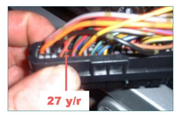
Pin #27 is the 5th from the left on the bottom row. It houses a yellow wire with a red stripe -- 1/2 of the Barbarian Jumper. Carefully remove this wire from the connector. Make sure you have the wire for pin 27 -- the other half of the jumper is only 2 pins away at 29, and we want to leave that half there.
