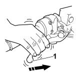
11.After the pulsating action has stopped in the brake lever, it is generated in the brake pedal "1" 0.5 second later and continues for approximately 2 seconds.
